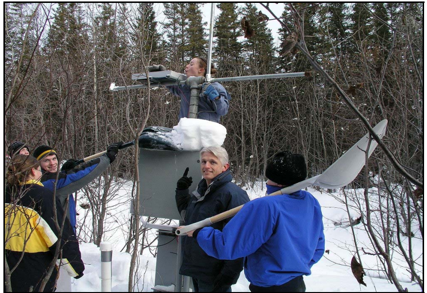
Figure 1: John Donaldson and Whitestone science class perform maintenance on a stream gaging station on Whitestone Creek. Campbell Scientific dataloggers collect stream temperature, conductivity, soil moisture, and stage information.
